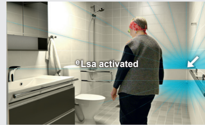
eLsa is activated when the person enters the room and is detected by the upper motion detector.
