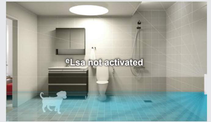
eLsa is not activated when a small animal such as a dog enters the room, since the upper motion detector will not be triggered in this case.
