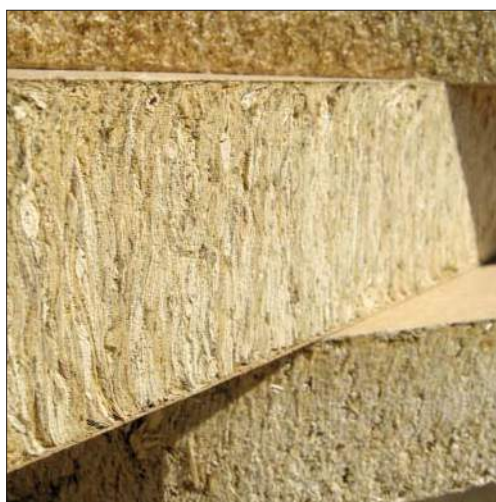
CROSS SECTION - S50 DURRA PANEL
